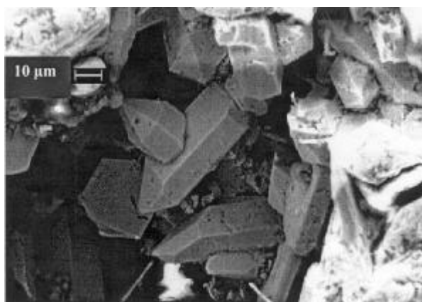
Figure 11. SEM of the fractured surface of Mo 5 Si 3 infiltrated at 1400°C for 30 min, well-developed hexagonal crystal like structures of MAS are seen.
